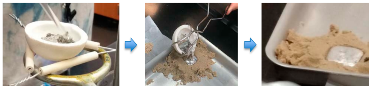
Figure 2. Metal casting using sand molds.
