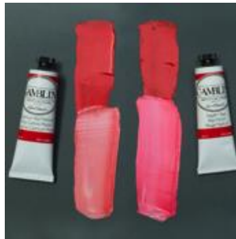
Figure.1 The mineral Cadmium Red Medium mixes with Titanium Zinc White (Left) Modern Naphthol Red mixes with Titanium Zinc White (Right)
